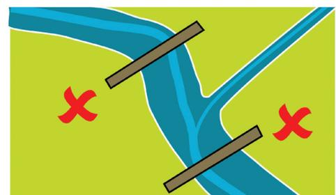
**Fig 8. Avoid locating dams either on bends or below inflows: where scour (pale blue line) is likely to become focussed close to one bank**
