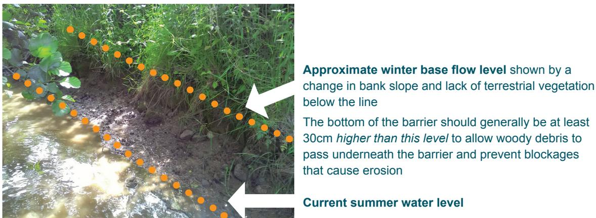
Fig 4. Estimating winter flow level from field evidence
