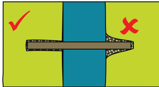
Using a narrow bucket allows logs to be slotted into their trench with minimal bank disturbance
