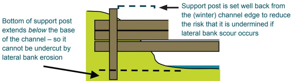
**Fig 7. Support posts: a belt and braces approach to ensure stability**
