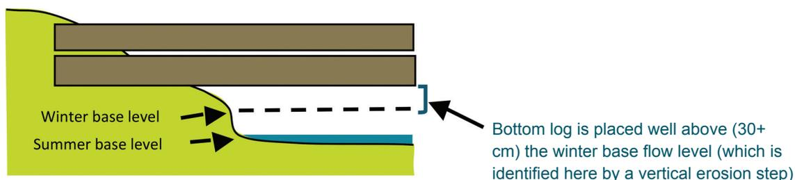
Fig 5. Ensure there is sufficient gap to let both winter flows and their debris, pass below the barrier unimpeded
