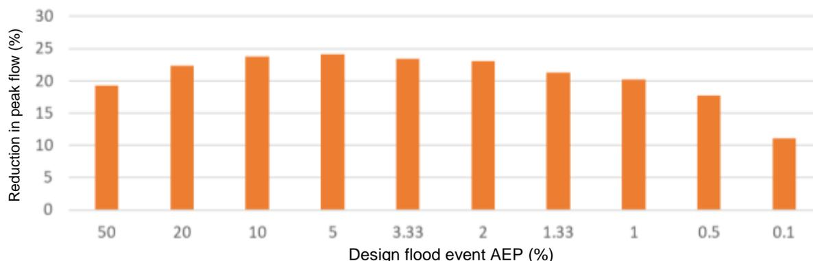
FIG. 2. Reduction in peak flow from the Eye Brook headwater catchment for a range of design flood events (AEP: Annual Exceedance Probability)
