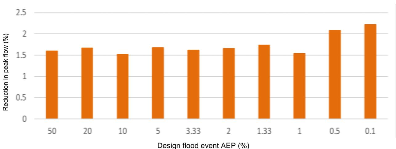
**FIG. 4. Reduction in peak flow 10 km downstream for a range of design events. Desynchronisation is the dominant effect on downstream flow and this is predicted to be retained even for the largest events.**
