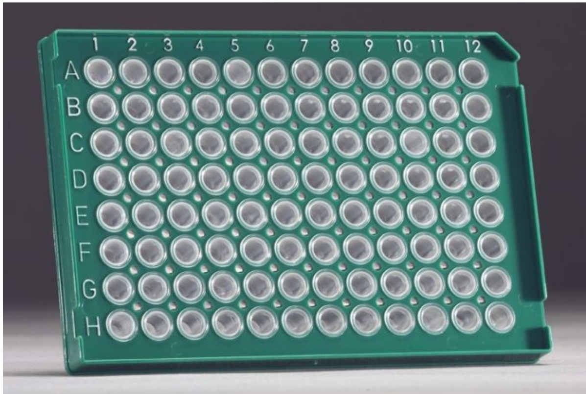
Figure 2.4. A PCR well plate. Replicates from a sample are arranged along a line of 12 wells (numbered 1-12). Samples are arranged in lines from A – H.
