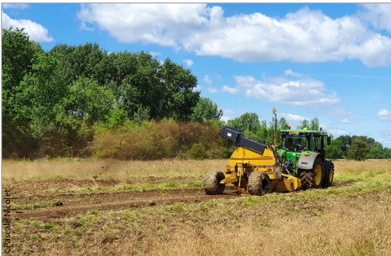
Scrapes creation using a rotary ditcher in the Waterstock IFA in 2019 has extended the feeding habitat of the nationally-declining Curlew. At that site, a fish refuge, a pond directly connected to the river, was also created in 2019, further enhancing the range of freshwater habitats at the site.
