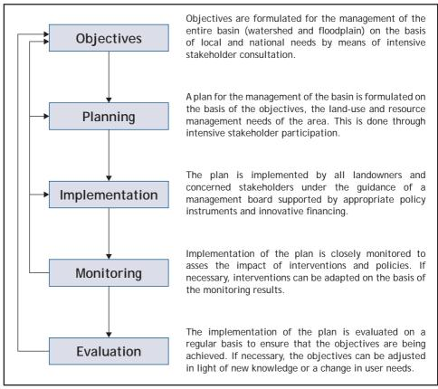
Figure 1: The iterative process of integrated basin management.
